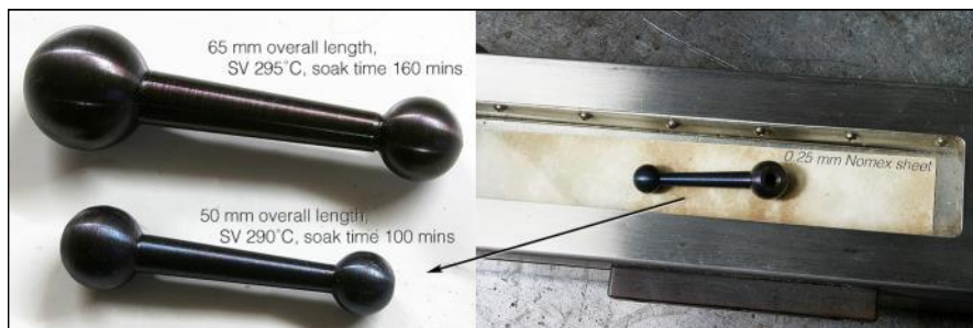
Figure 29: Machine tool ball handle bluing trials. No lidded chamber was used, but the Nomex sheet coupled with the handles' large thermal mass and long soak time did contribute significantly to the even colouration
