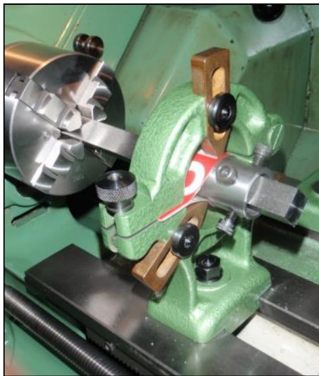
2. Well oiled card can help prevent work being damaged by the jaws of the fixed steady.
