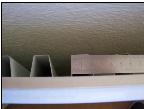
Photo. 4. A 'Type 11' domestic single panel domestic heating radiator.
