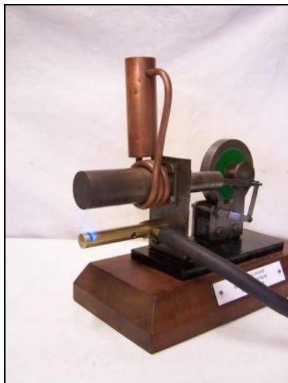
Photo. 1. The engine with the new propane burner and the original copper cooling coil.
