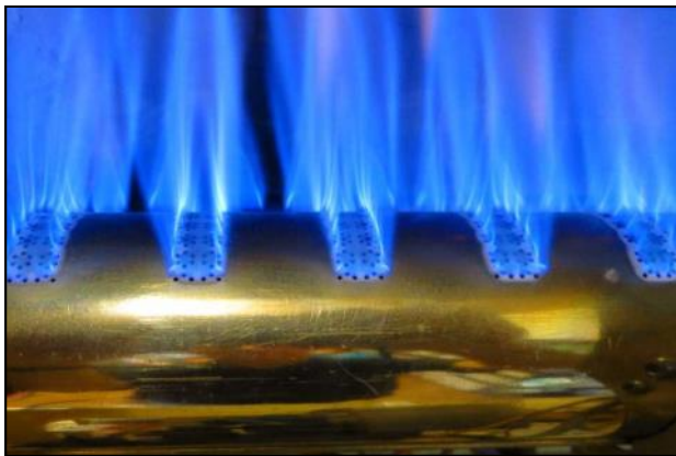
Photo. 2. A typical burner for a non-condensing central heating boiler showing the gaps between the flames. (Photo courtesy of Paul Huzar, Boiler Services Ltd, Hawkchurch, Exeter).
