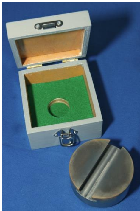
Jonathan Tickner's solid toolpost for his Boxford lathe with its custom box.
