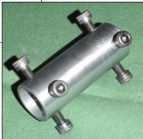
1. A simple cathead made from steel tube and fitted with eight screws.
