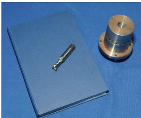
Joe Sissons showed three items including a slot drill re-sharpened on a Worden tool and cutter grinder, a bearing and screw assembly for a standing press for bookbinding and a copy of The Amateur's Lathe by L.H. Sparey re-bound using the press.
