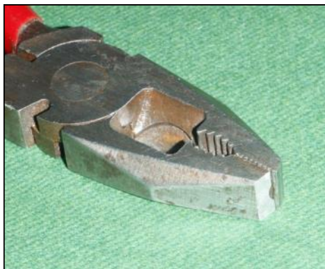
3. The pliers were also provided with one shortened jaw (the grooved one).
