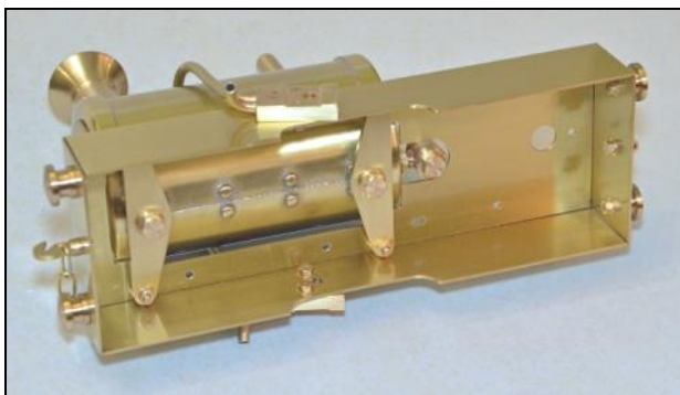
14: Boiler assembly fitted to chassis.
