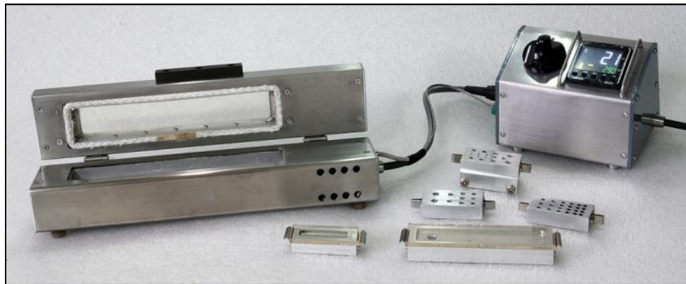
Figure 6: The author's PID controlled bluing box.
