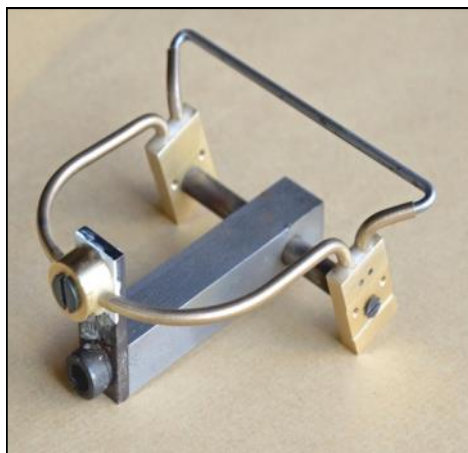
11: An armature was used to support the cylinder steam supply pipework for silver brazing.
