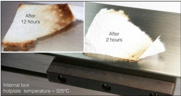
Figure 8: Ignition trial on a piece of kitchen paper.
