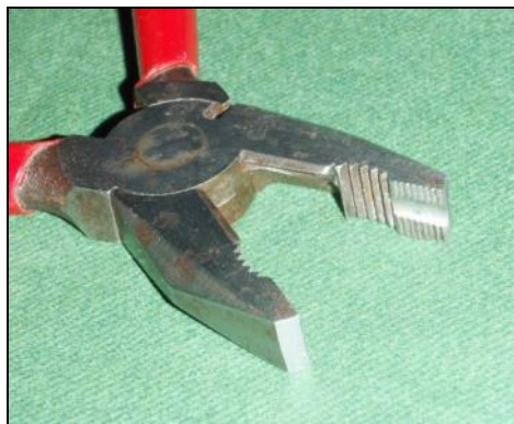
2. The pliers' jaw modified by adding a groove.
