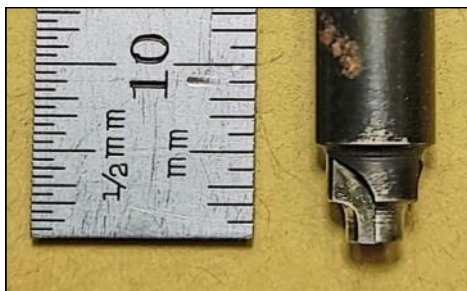
8: Silver steel corner rounding cutter.
