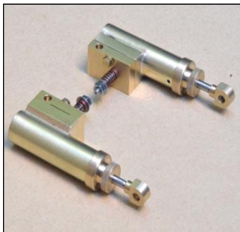
10: Single-acting oscillating cylinder assemblies.
