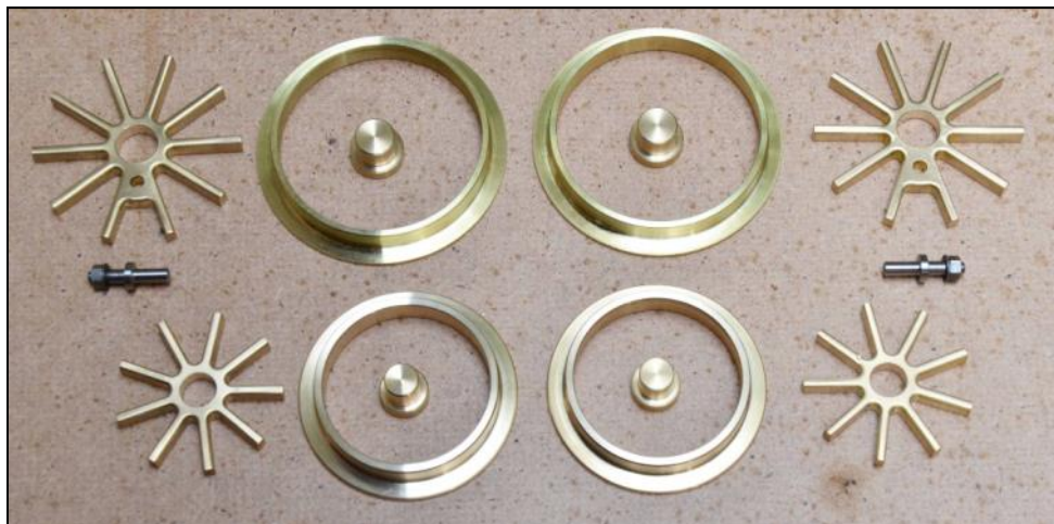
9: Driving wheel rims, bosses, spokes and crankpins (top); leading wheel rims, bosses and spokes (bottom).
